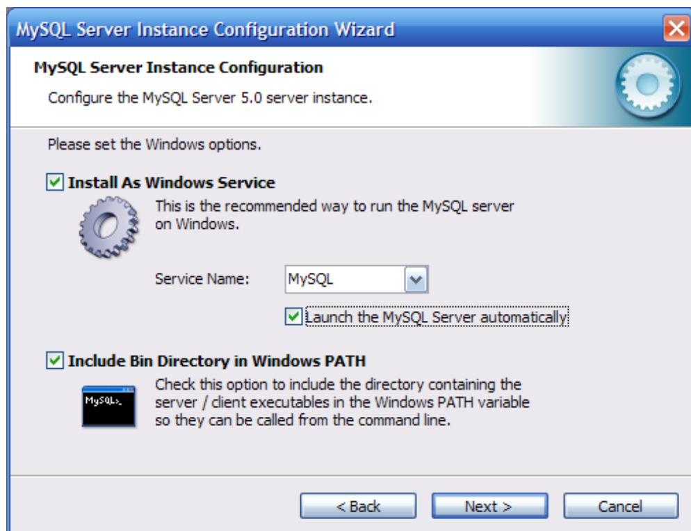
Figure 9. Windows options page of the MySQL Server Instance Configuration Wizard
